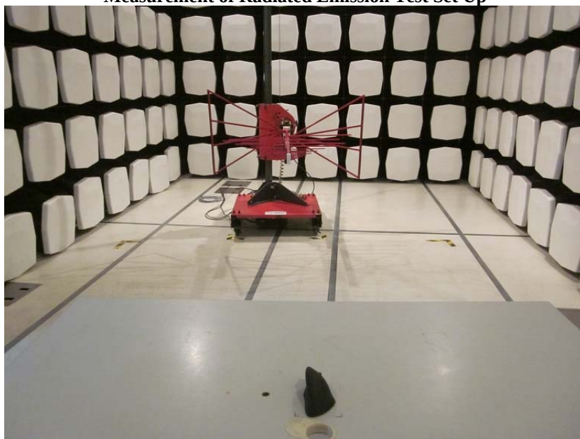
Measurement of Radiated Emission Test Set Up
