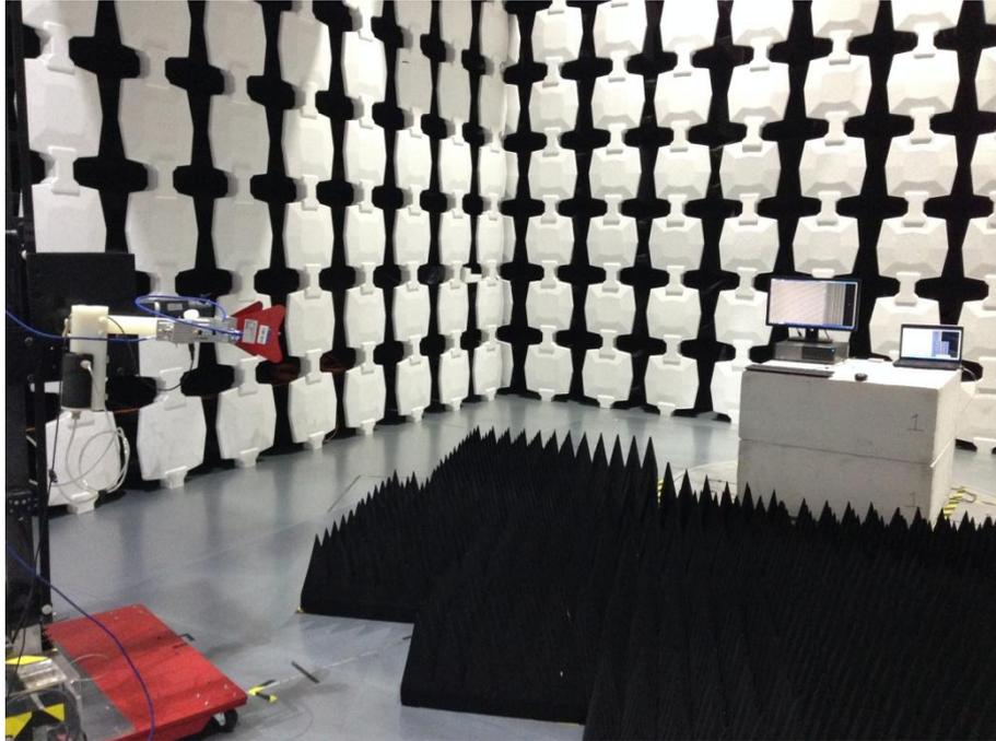
Description: Front view of Radiated Emission Test Setup (30-1000MHz)
