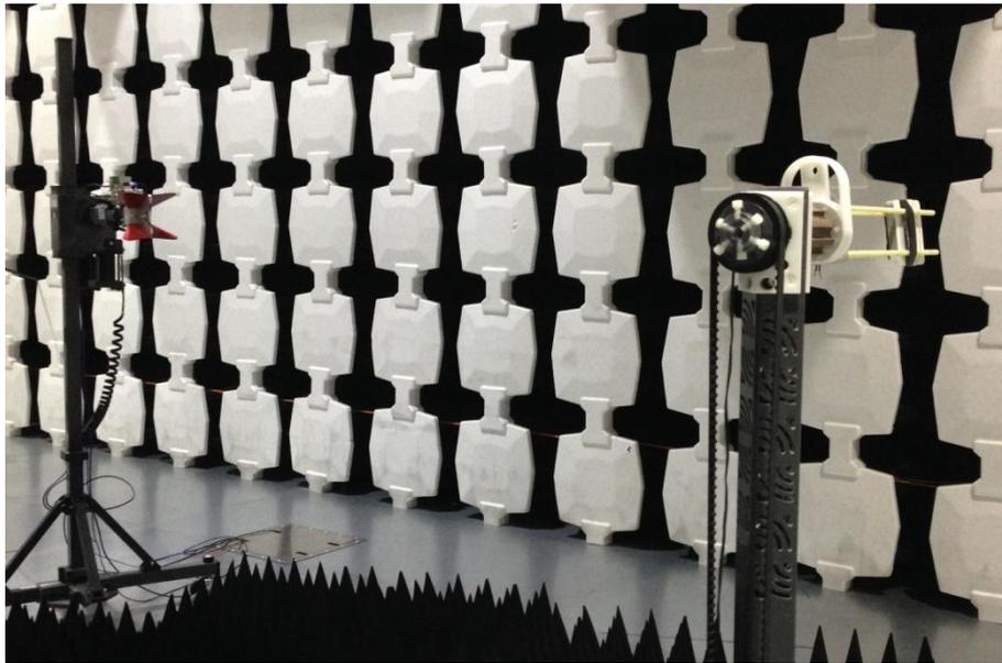
Description: Substitution Antenna for EIRP Test
