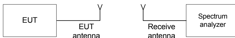
Figure 7.2.1 Carrier frequency separation test setup
