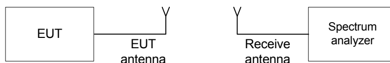
Figure 7.1.1 The 20 dB bandwidth test setup
