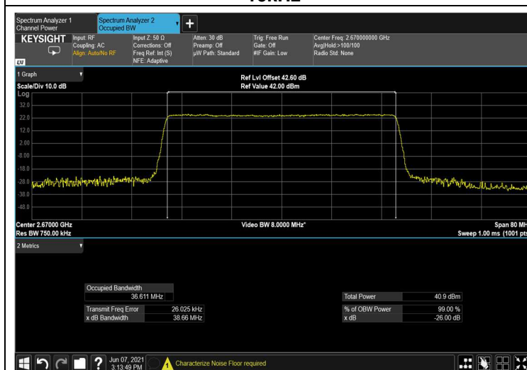
Figure 175: output 256QAM 40MHz B.W.; 2670.0MHz, 60kHz
