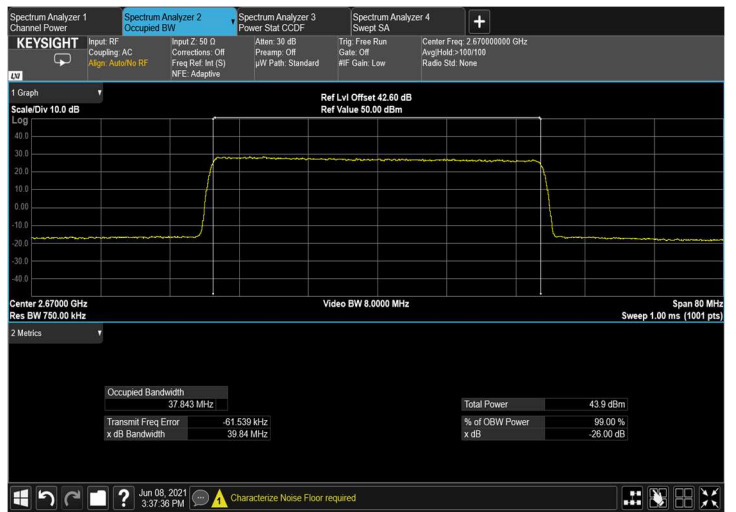
Figure 159: output 64QAM 40MHz B.W.; 2670.0MHz, 30kHz
