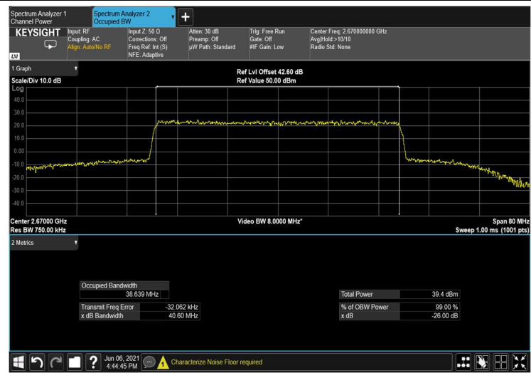
Figure 188: output QPSK 40MHz B.W.; 2670.0MHz, 15kHz
