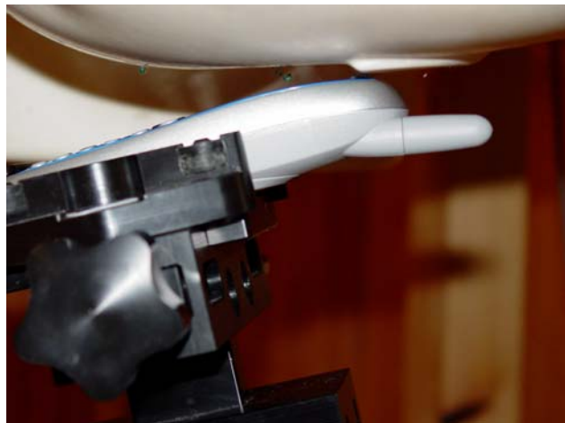
Figure 11.3 phone against the head (left tilt position)
