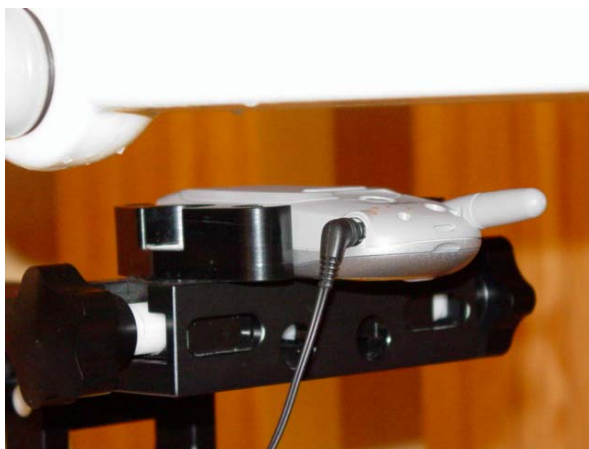
Figure 11.6 body SAR set-up (with 22.5mm air separation)
