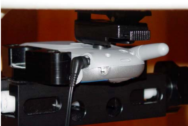
Figure 11.4 body SAR set-up (with belt clip)
