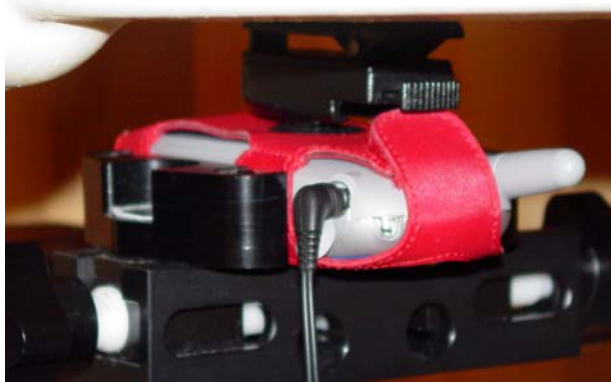
Figure 11.5 body SAR set-up (with leather case)
