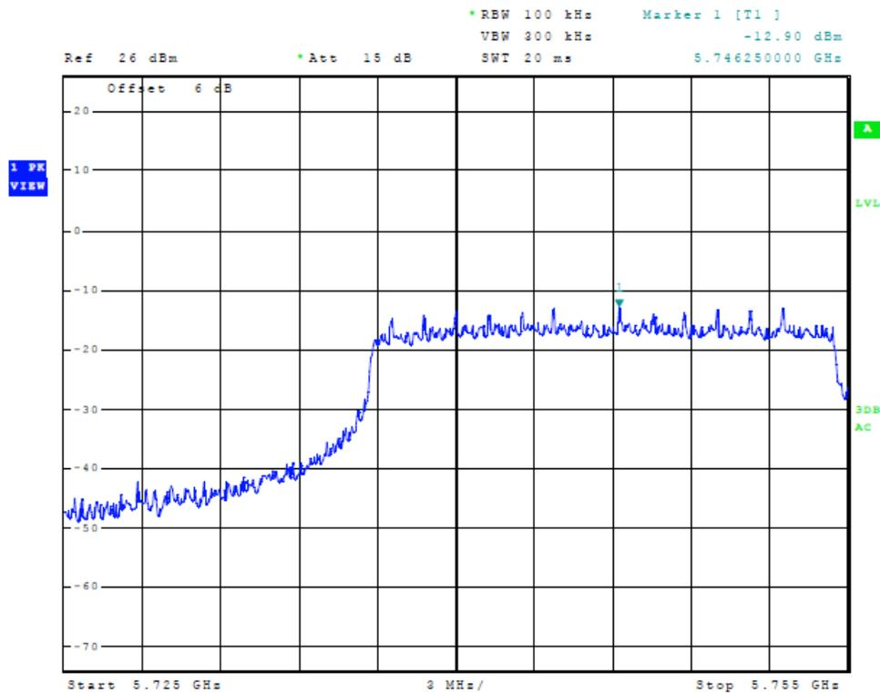
Figure 8 Plot of Transmitter Low Band Edge (40 MHz Channel)
