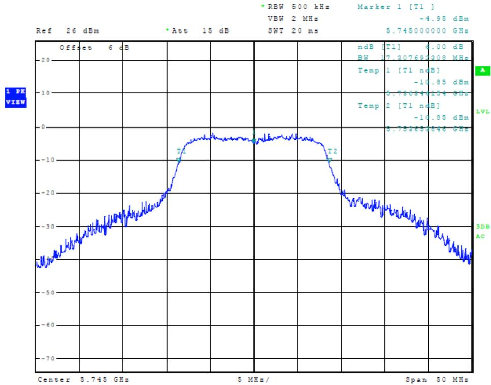
Figure 11 Plot of Transmitter Occupied Bandwidth (20 MHz Channel)
