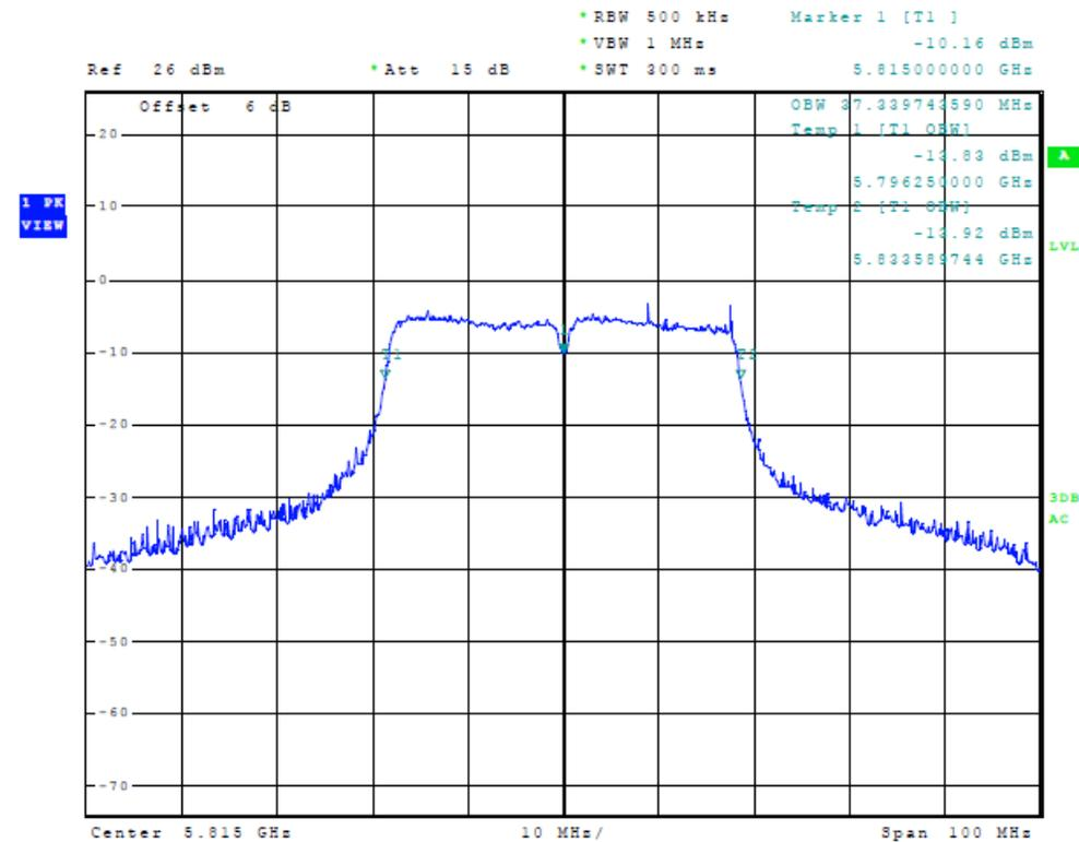
Figure 12 Plot of Transmitter Occupied Bandwidth (40 MHz Channel)
