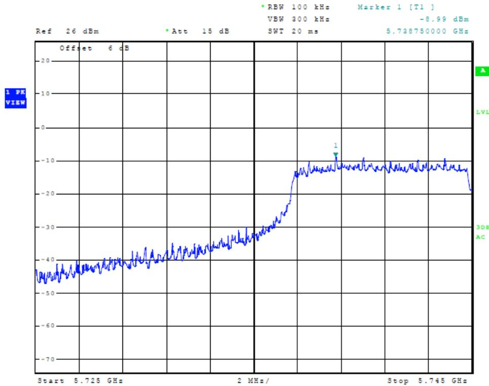
Figure 7 Plot of Transmitter Low Band Edge (20 MHz Channel)
