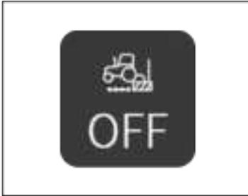
Draft mode icon shows the current mode of the vehicle. If Draft mode icon is “ON”, the vehicle will operate in Draft mode. When the engine is off, “OFF” is shown.
