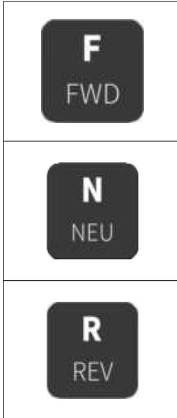
Shuttle Direction icon shows the current direction of the shuttle lever.
