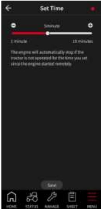
If the machine is not in operation mode within the specified time, the remote start will automatically shut down for safety reasons.
