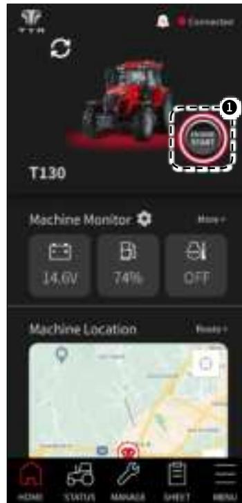
While the engine is off, 'Engine Button'<sup>①</sup> is displayed in black with the text 'ENGINE START'. Remote engine start can be executed with PIN code.
