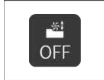
Depth mode icon shows the current mode of the vehicle. If Depth mode icon is “ON”, the vehicle will operate in Depth mode. When the engine is off, “OFF” is shown.
