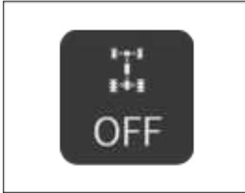
4WD icon shows the current mode of the vehicle. If 4WD icon is “ON”, the vehicle will operate in 4-Wheel Drive mode. When the engine is off, “OFF” is shown.
