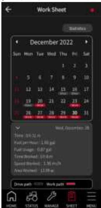
When the machine starts, it shows 'Drive' in gray. Under work conditions, it turns to 'Work' in red.
