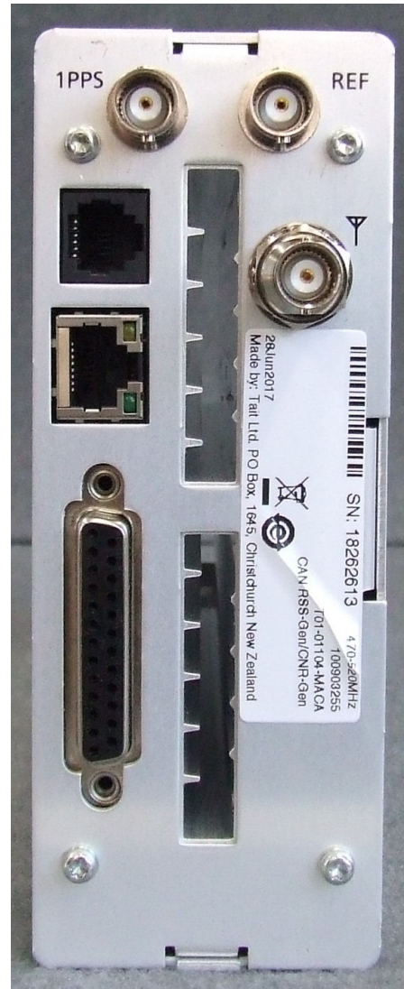
Photograph 07: Reciter module – Rear panel
