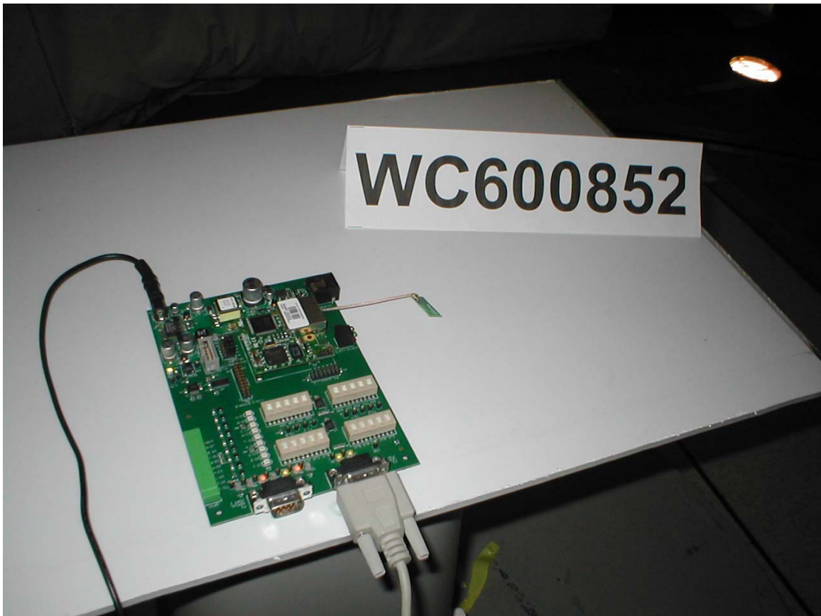
Test Set-up photo, radiated emissions
