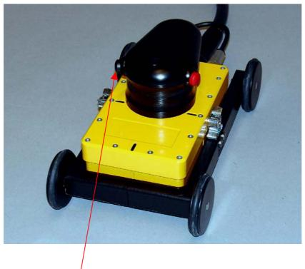
Kill switch, must be constantly depressed. When switch is released, pulse generator will cease firing pulses within 10 seconds.
