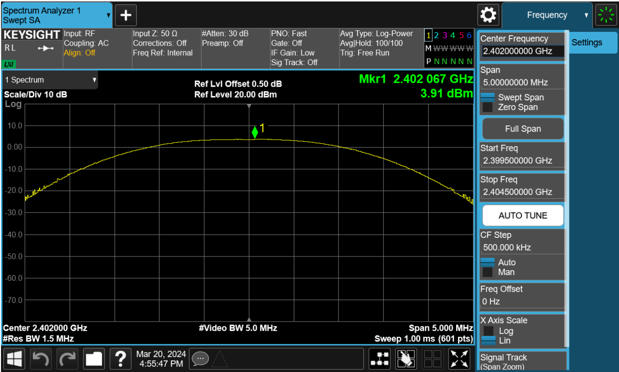
Figure 2: Peak Output Power, 2440MHz, BLE-1Mbps
