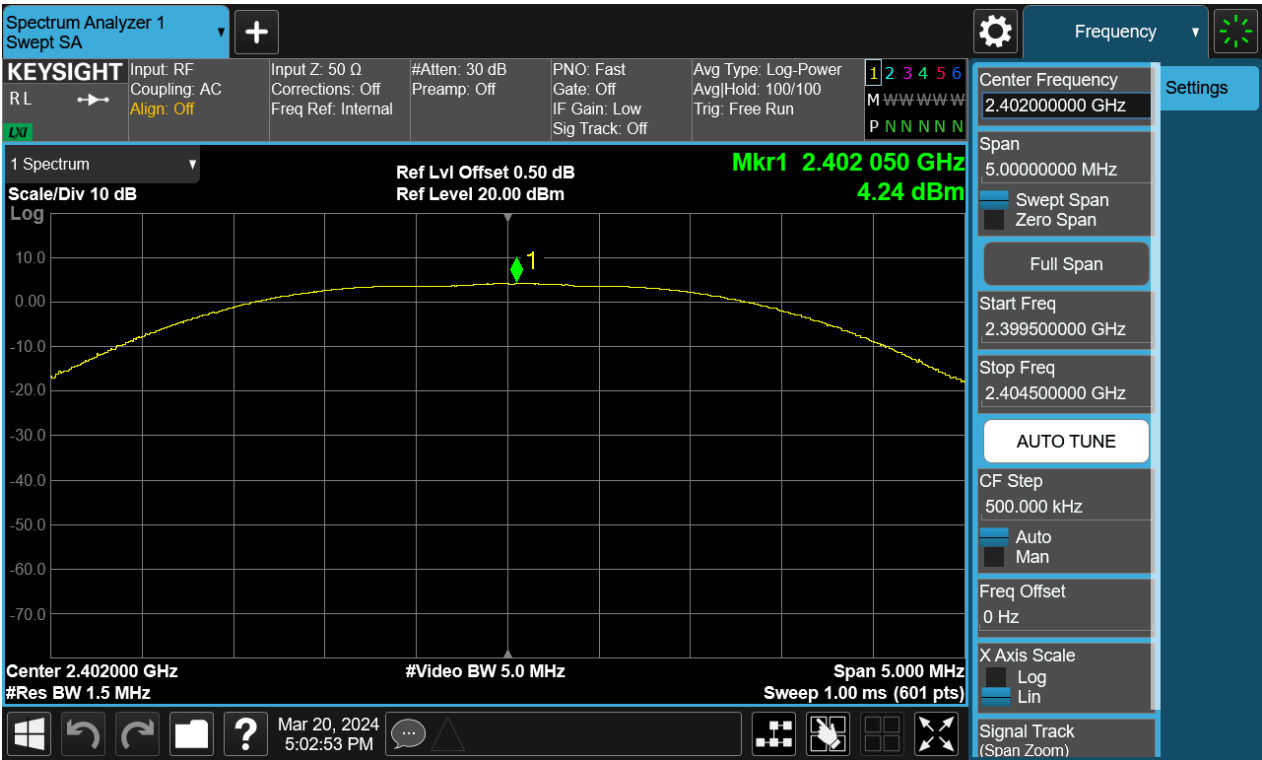
Figure 4: Peak Output Power, 2402MHz, BLE-2Mbps
