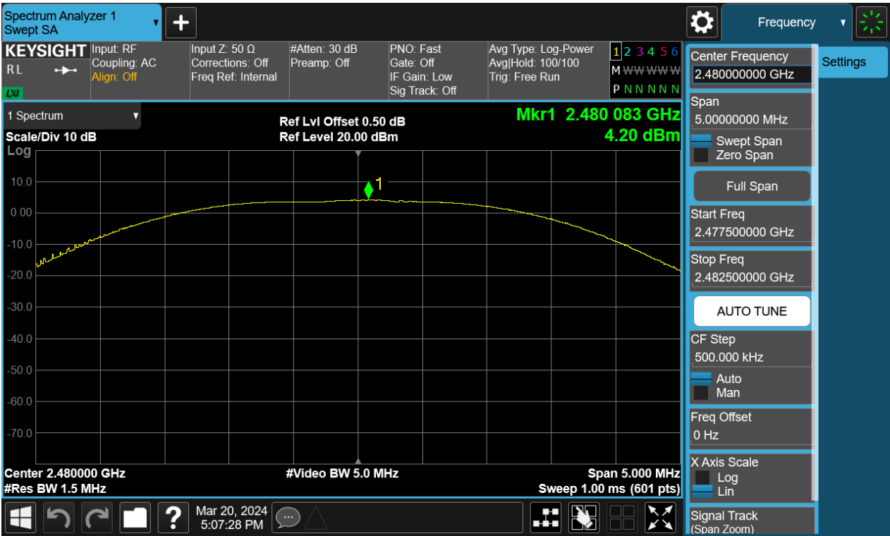
Figure 6: Peak Output Power, 2480MHz, BLE-2Mbps
