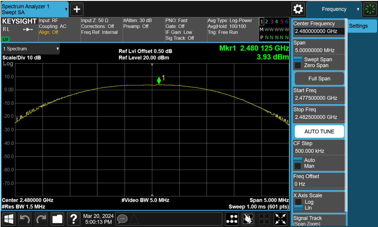
Figure 4: Peak Output Power, 2402MHz, BLE-2Mbps
