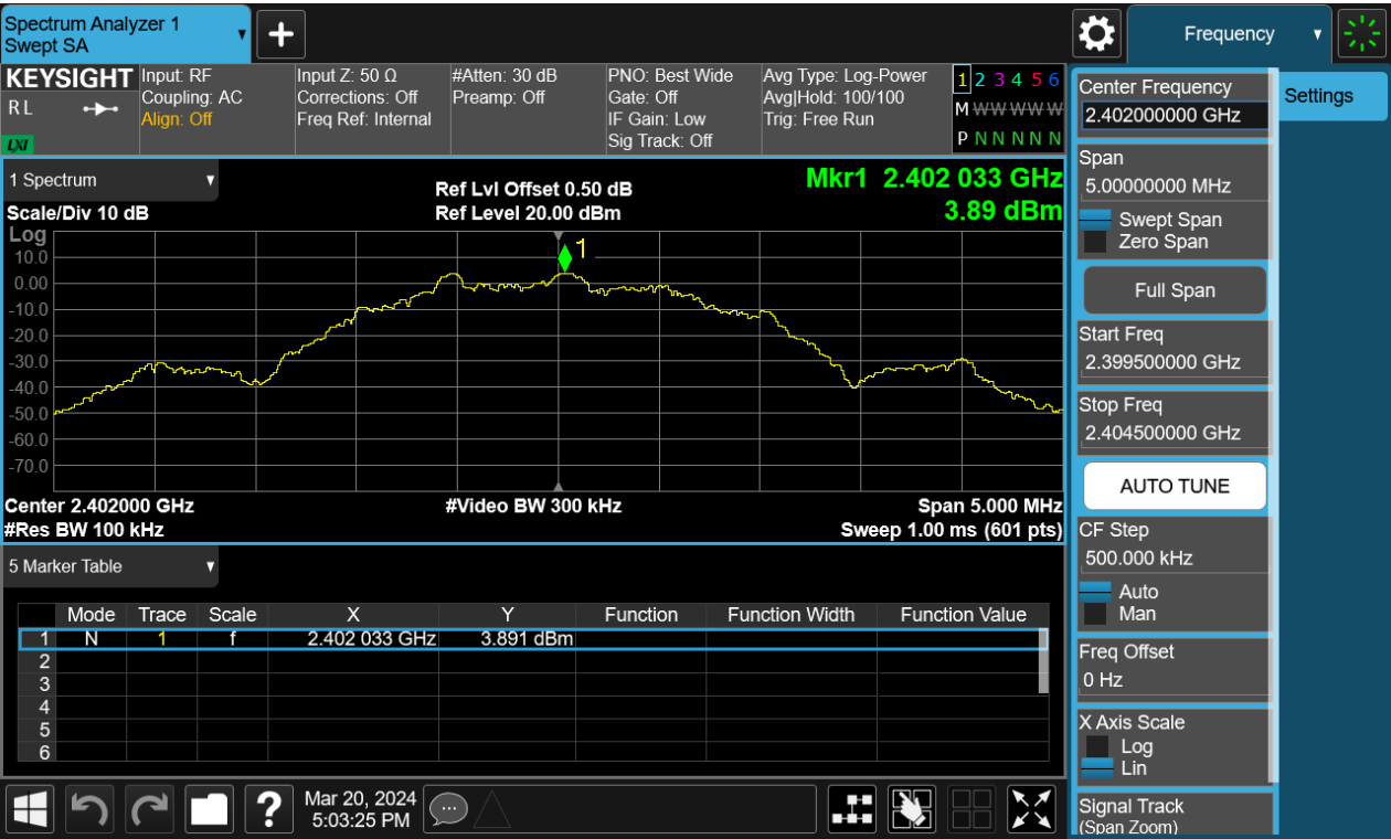
Figure 22: Conducted Spurious Emission & Authorized-band band-edge, 2402MHz, BLE-2Mbps Carrier Level
