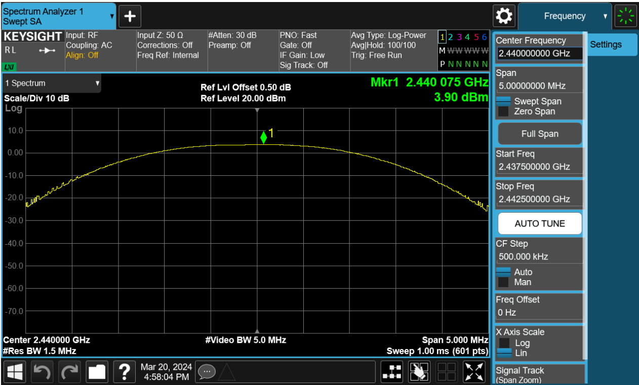
Figure 2: Peak Output Power, 2440MHz, BLE-1Mbps
