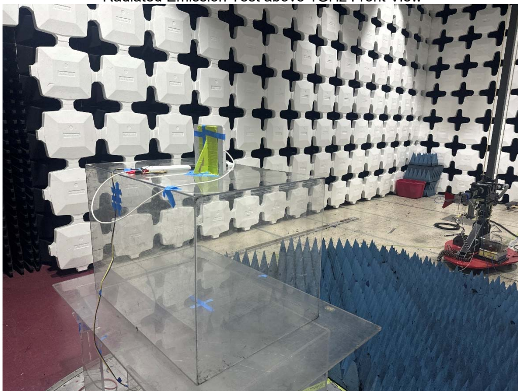
Radiated Emission Test above 1GHz Rear View
