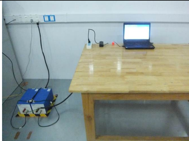
Conducted Emissions Test Setup Front View
