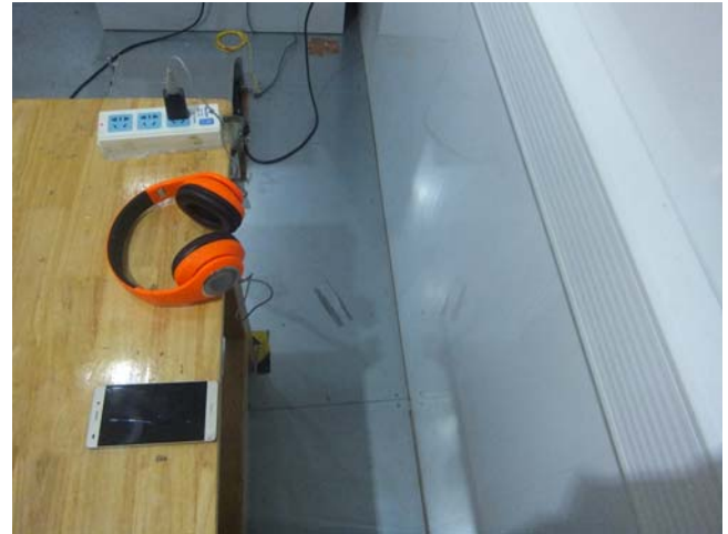
Conducted Emissions Test Setup – Side View
