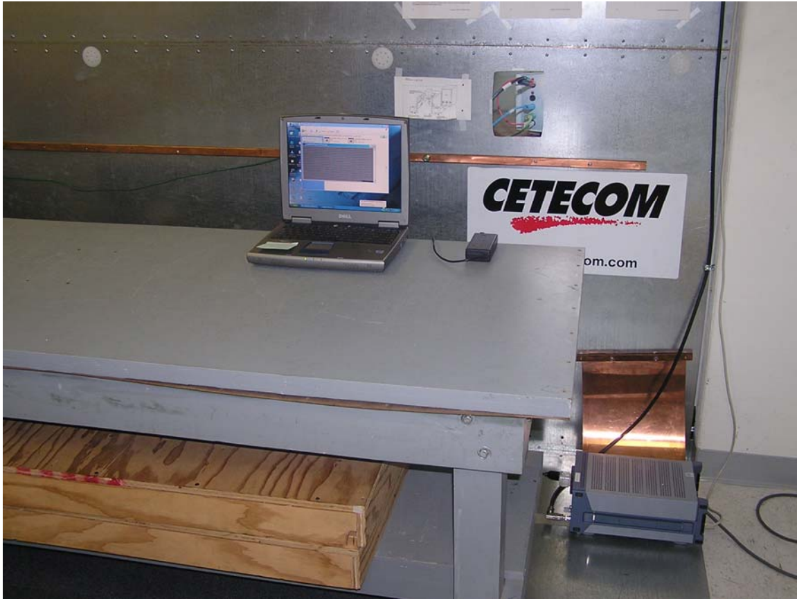
Test setup – AC Line conducted measurement
