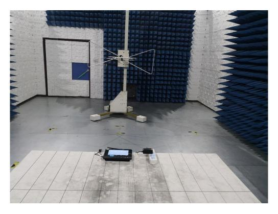
FCC RADIATED EMISSION TEST SETUP ABOVE 1GHZ
