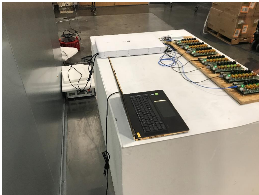
Photograph 5: Back View Test Set Up Conducted Emissions
