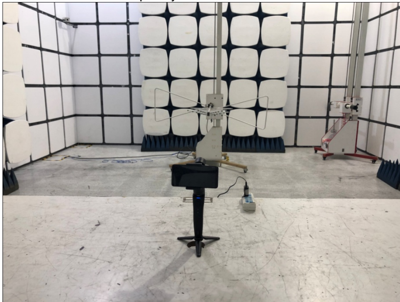
Radiated Spurious Emissions Test Frequency From 30MHz-1000MHz
