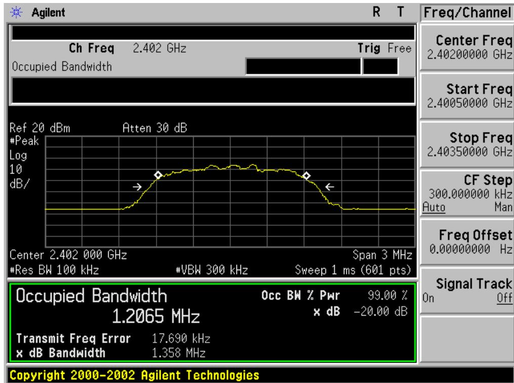
TEST PLOT OF BANDWIDTH FOR MIDDLE CHANNEL
