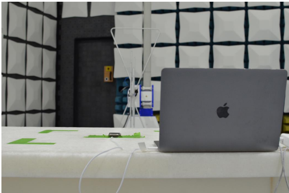
Figure 15: 30MHz-960MHz Test Setup (Rear View)
