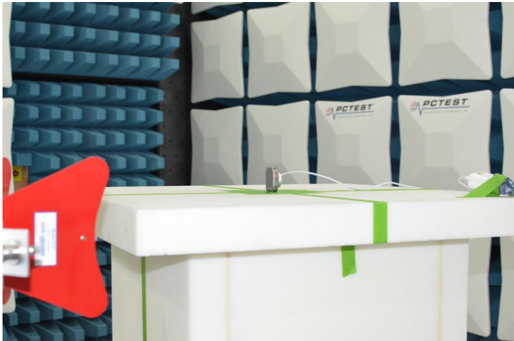
Figure 7: Above 960MHz Test Setup
