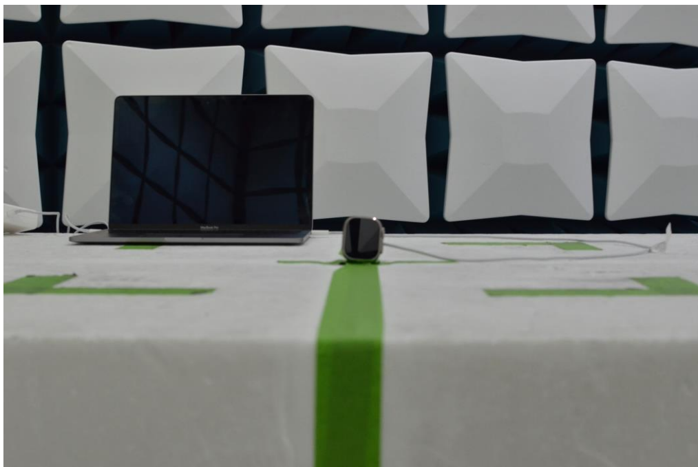
Figure 18: 30MHz-960MHz Test Setup (Front View)
