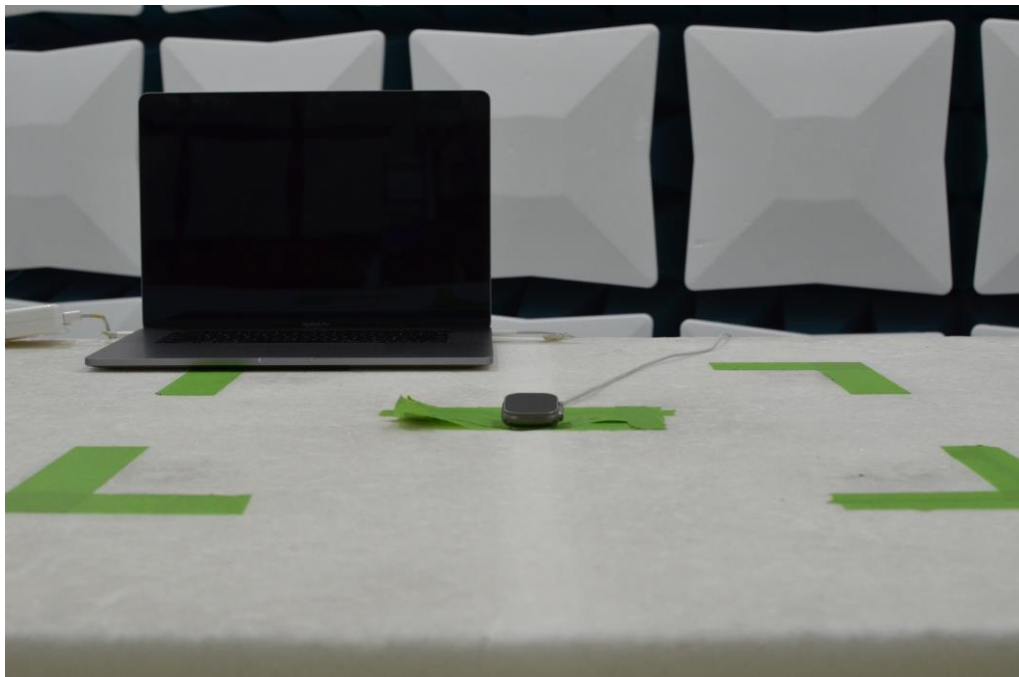
Figure 14: 30MHz-960MHz Test Setup (Front View)
