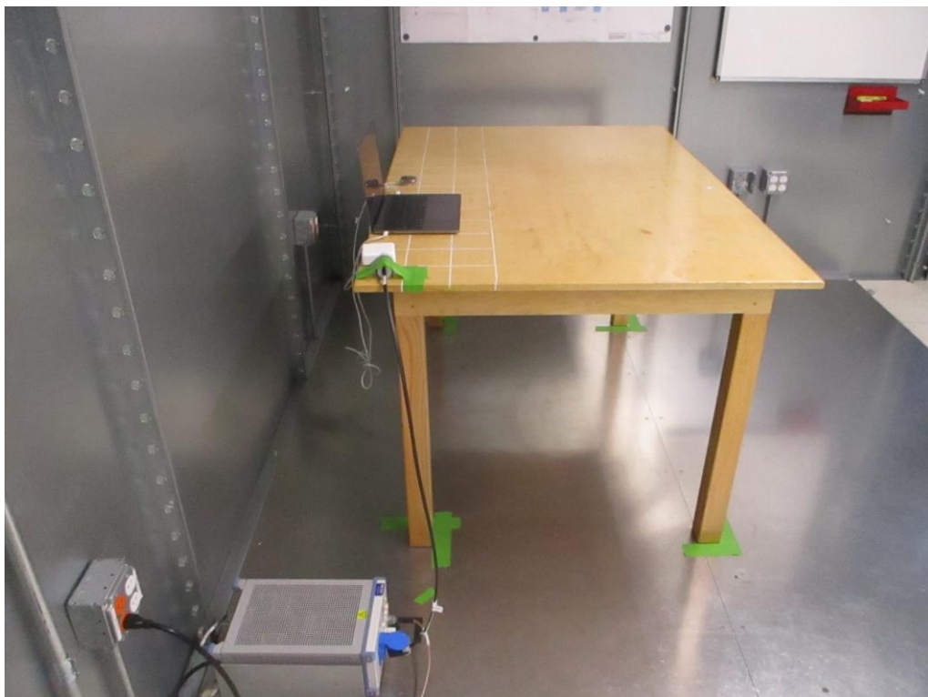
Figure 4: AC Line Conducted Emissions (Side View)
