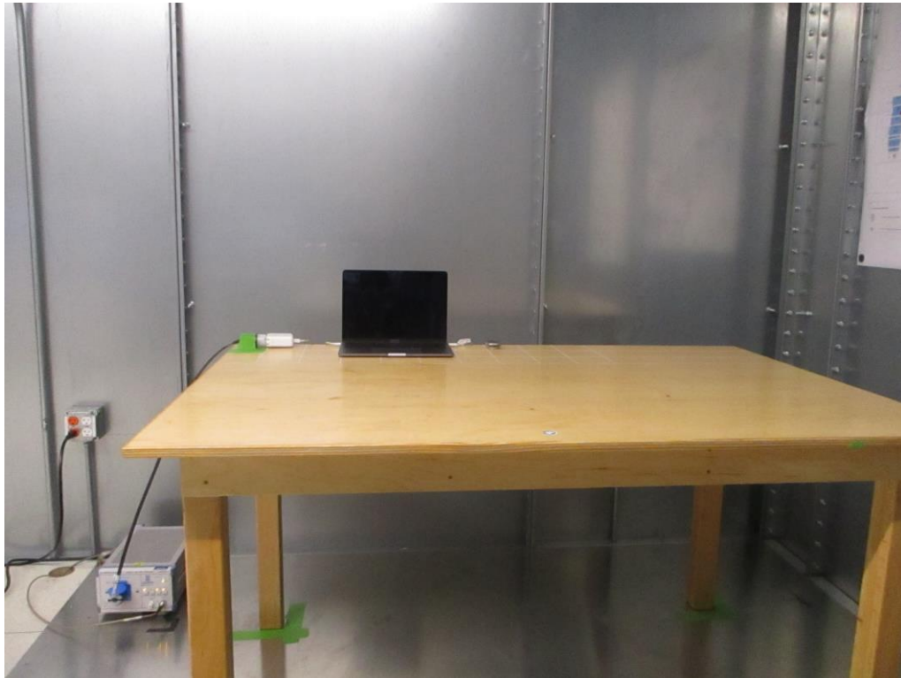
Figure 3: AC Line Conducted Emissions (Front View)
