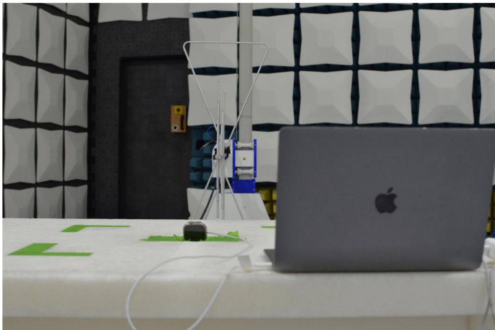
Figure 17: 30MHz-960MHz Test Setup (Rear View)
