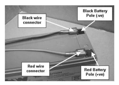
• **ATTENTION**: Make sure the battery connector wires are connected to the same color of the battery pole i.e. black color wire connector connected to the black color battery pole (-ve) and red color wire connector connected to the red color battery pole (+ve).
