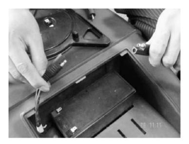
• Remove the battery connector from the HMMWV M1045A2 TOW Missile Carrier harness connector.
