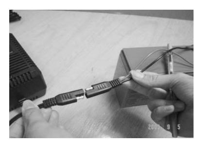
• Plug the charger connector into the battery connector.
