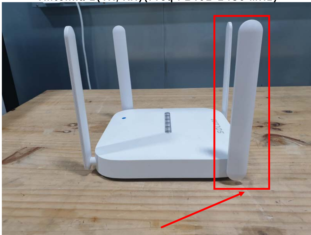
Antenna 2(TX, RX)(Freq : 2402-2480 MHz)
