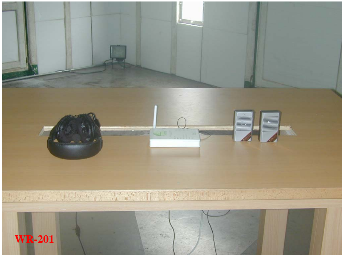
Photo 1: Radiated Emission Test set-up photo
