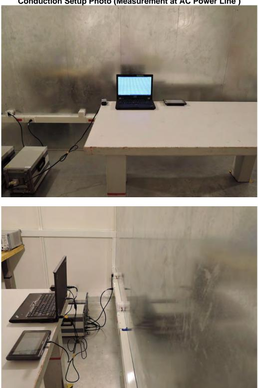
Conduction Setup Photo (Measurement at AC Power Line)
