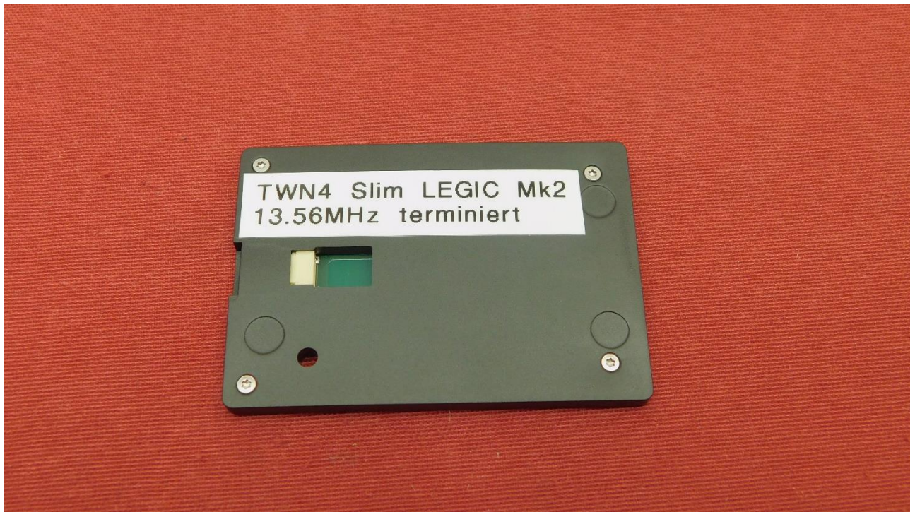
Picture 3: EUT used to perform AC power line re-test in mode 2 (RF chip is terminated with a dummy load) – bottom view
