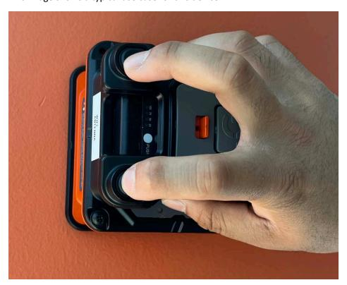
**Antenna 2 Location:** The second antenna is located at the rear side under the battery well. (See white sticker). It is approximately 29mm away from the bottom of the top cover. The hand will rest at least a couple mm higher than the 29mm distance in any way the user holds and use the device.
