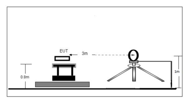
(B) Radiated Emission Test-Up Frequency 30MHz~1GHz
