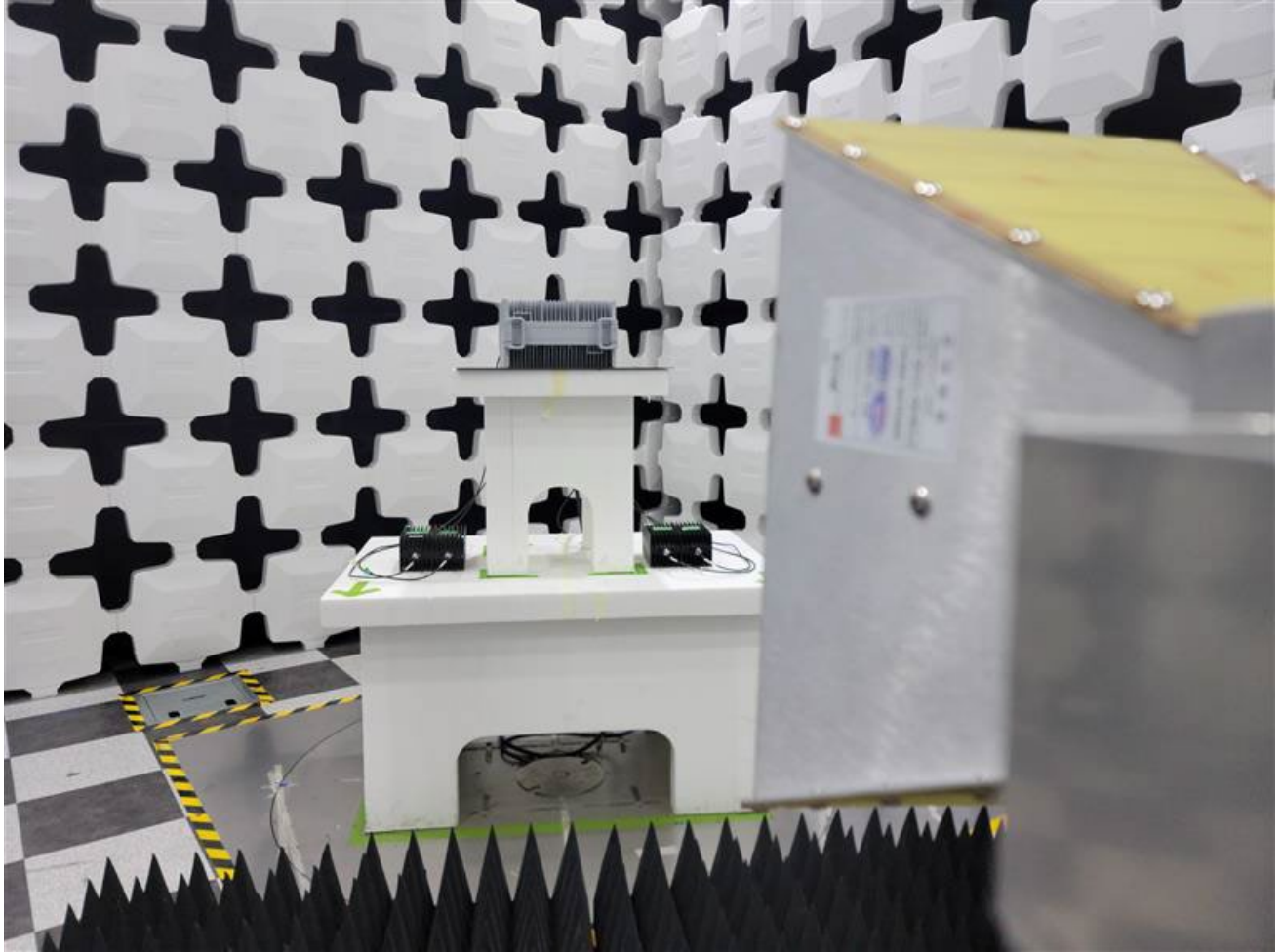
Above 1GHz Test Instrument & Measurement Setup > 1GHz
