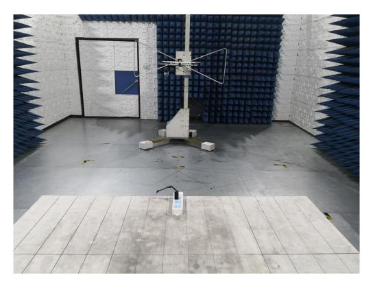
RADIATED EMISSION TEST SETUP ABOVE 1GHZ
