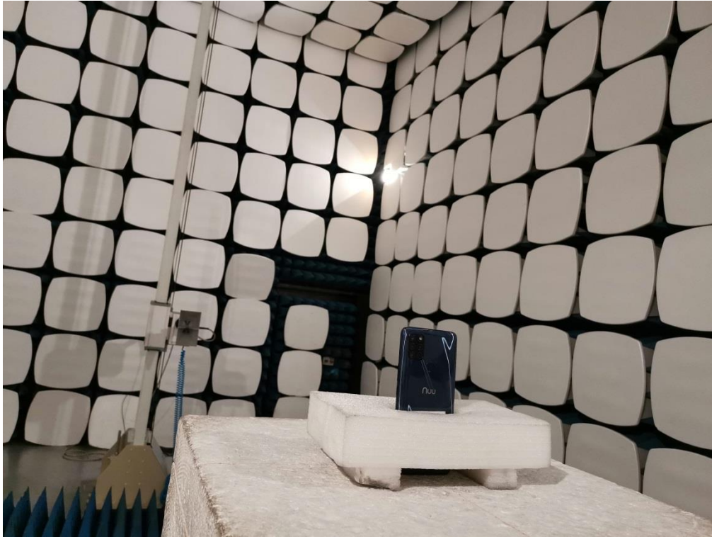
Radiated Spurious Emission Below 1GHz
