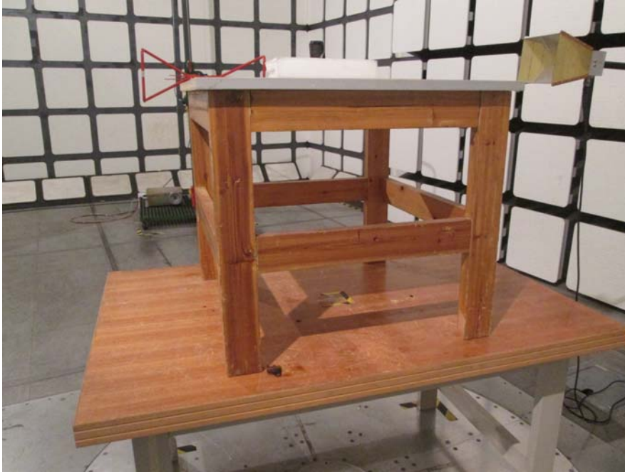
Radiated Emissions Test View (Below 1 GHz)
