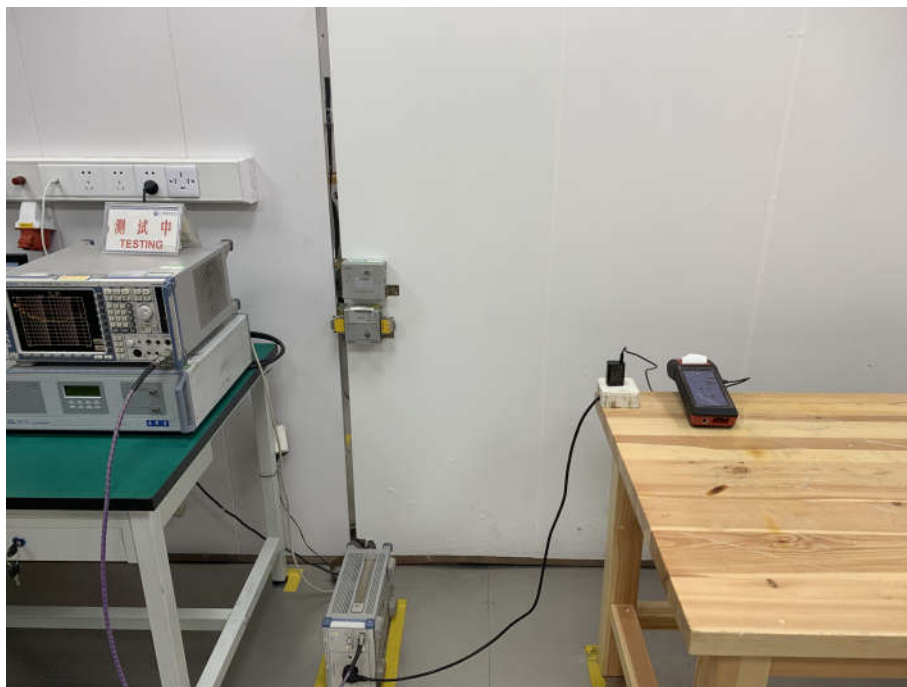
Conducted Emissions Test Setup
