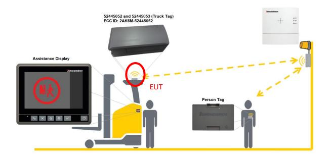
The product family FCC ID: 2AK6M-52445052 (52445052 and 52445053) is connected to the user interface (Assistance Display) via cable because it has its own user interface.
