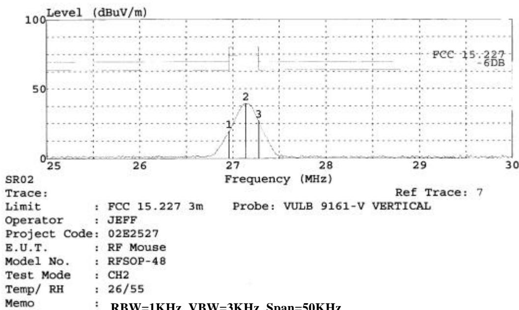
**6.3 Bandwidth requirement Mode : Operation frequency: 27.045 MHz, CH2**
