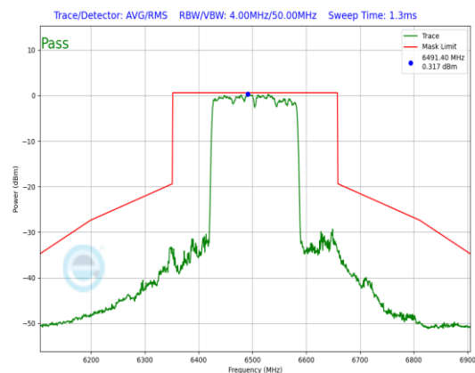
Plot 7-872. In-Band Emission Plot CDD Diversity Antenna 1b (160MHz 802.11ax RU996x2 (UNII Band 6) – Ch. 111)
