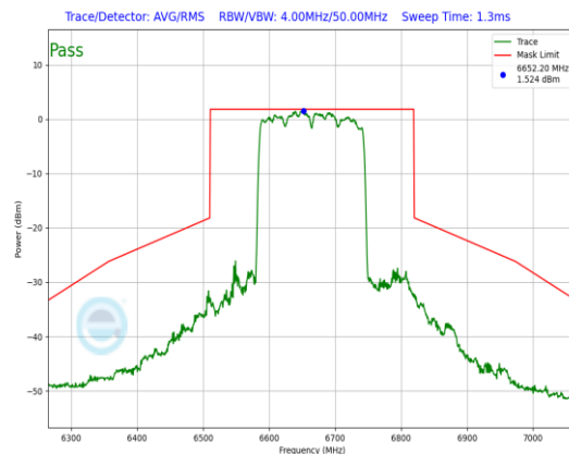
Plot 7-888. In-Band Emission Plot CDD Diversity Antenna 1b (160MHz 802.11ax RU996x2 (UNII Band 7) – Ch. 143)
