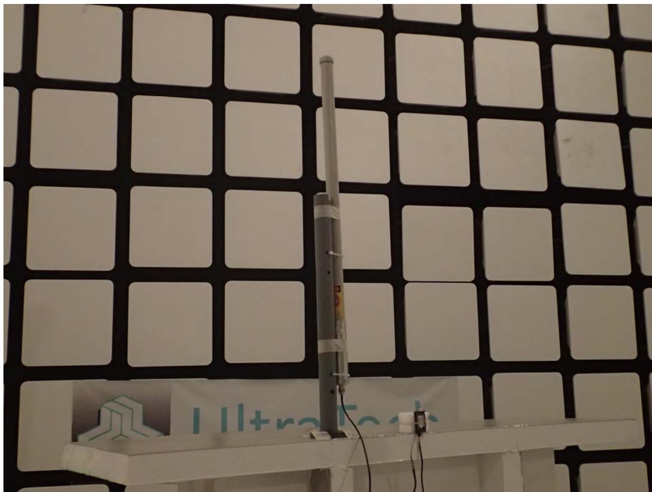
Radiated Emissions @ 3 m EUT with 15 dBi Omni Directional Antenna, Orthogonal Position 3
