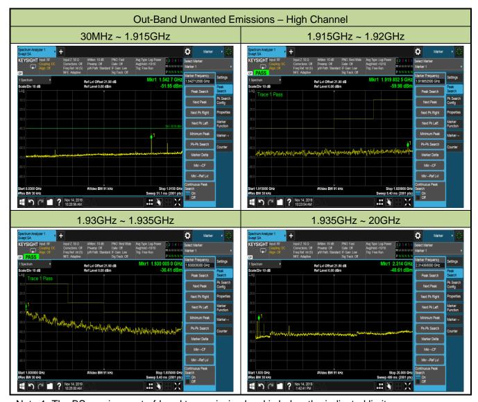
Note 1: The BS spurious out-of-band transmission level is below the indicated limit.
