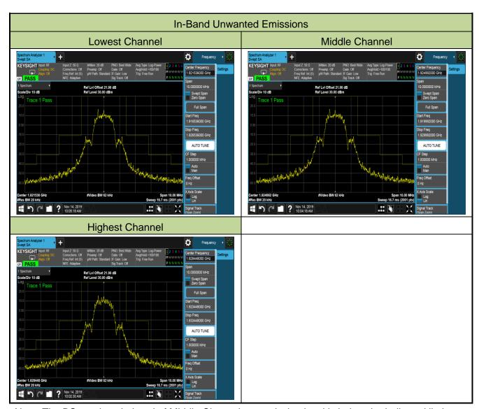
Note: The BS spurious in-band of Middle Channel transmission level is below the indicated limit.
