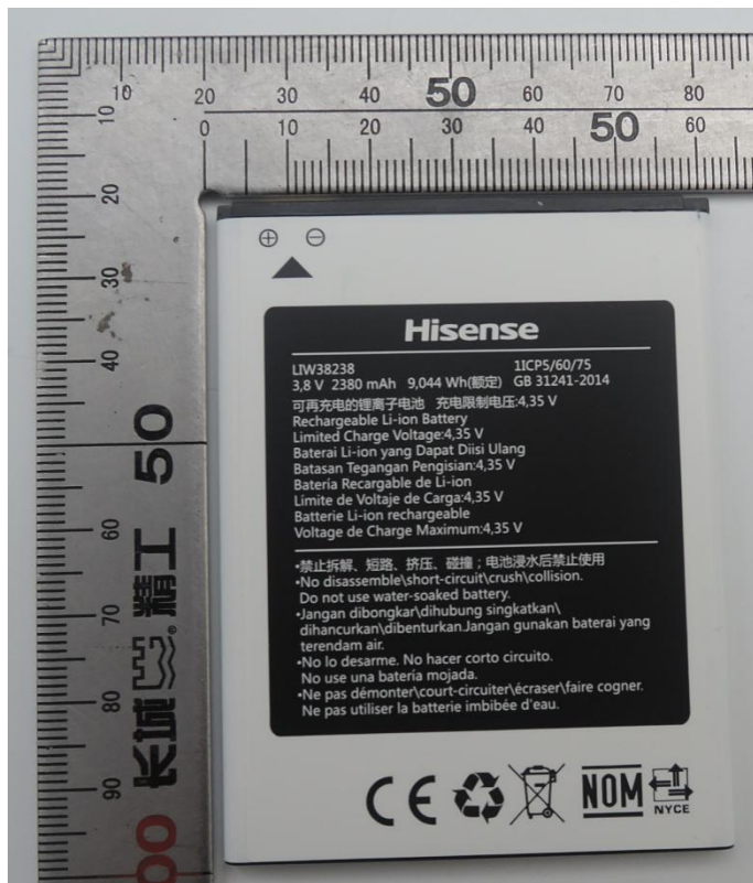
The battery view (Li3822T43P3h716043)
