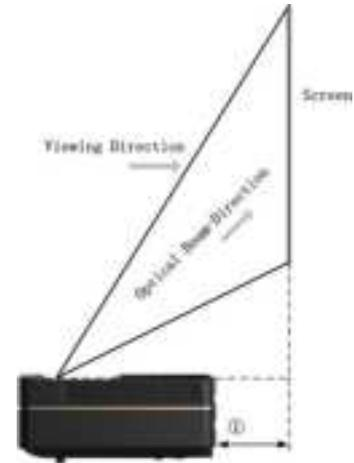
Fig. 12 Installation distance
