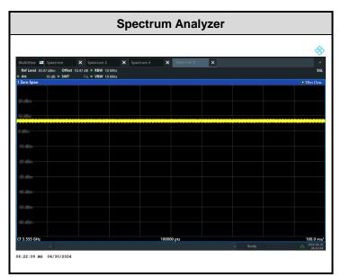
Note: The duty cycle value is 100%; therefore, the 10log(1/duty cycle) factor would not be taken into account when computing the average power during continuous transmission.
