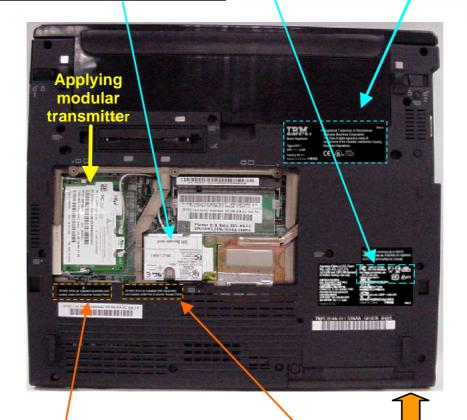
TX FCC ID for an installed transmitter card located under this Customer Access Panel
