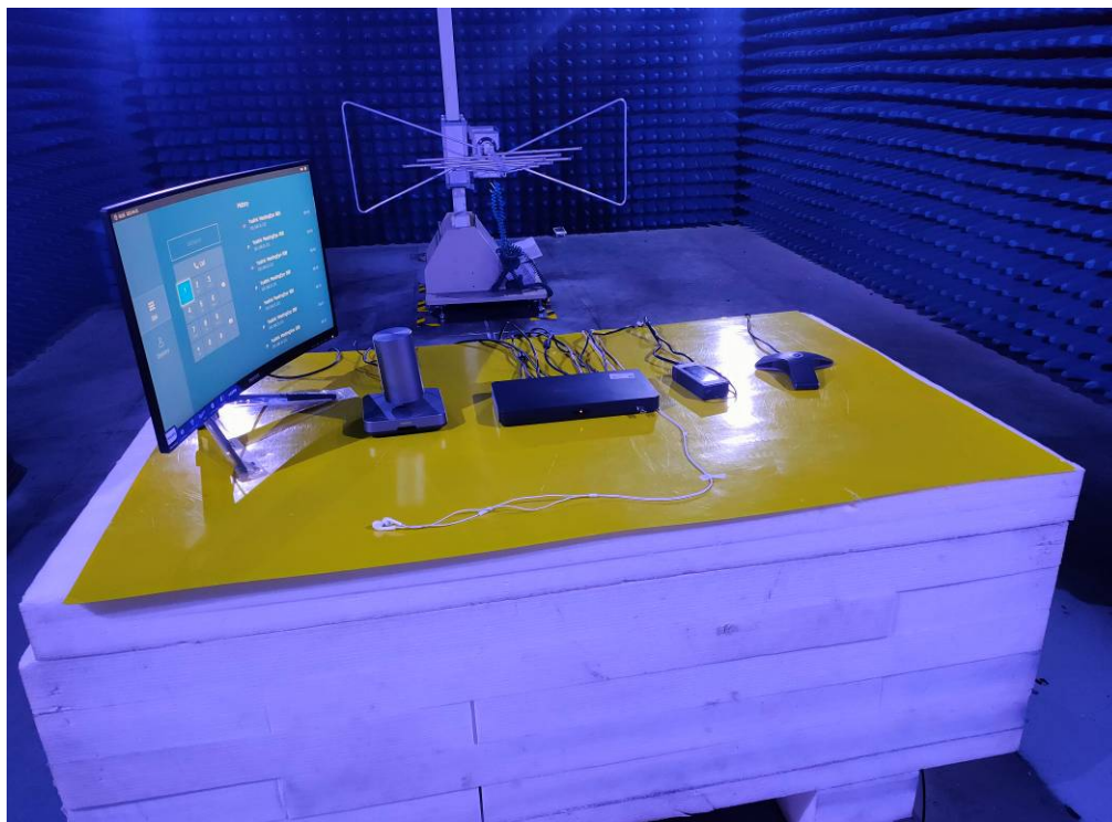
Photo of Radiated Emission Measurement (Above 1G)
