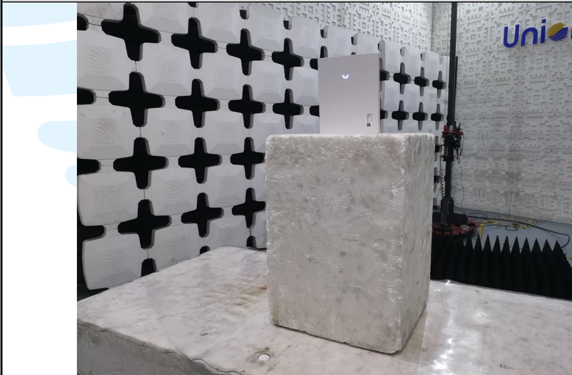
Radiated emission Test Setup (Above 1 GHz)
