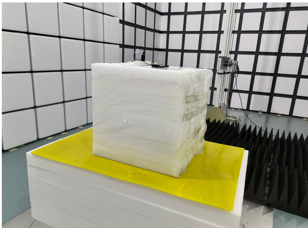
Photo of Radiated Emission Measurement (Above 1G)
