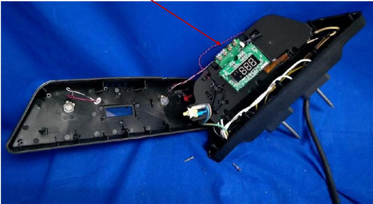
The Saber (Weber Connect) design is a single board. The module electronics are contained in the 1DX chip and the antenna are identical. The antenna match is also identical.
