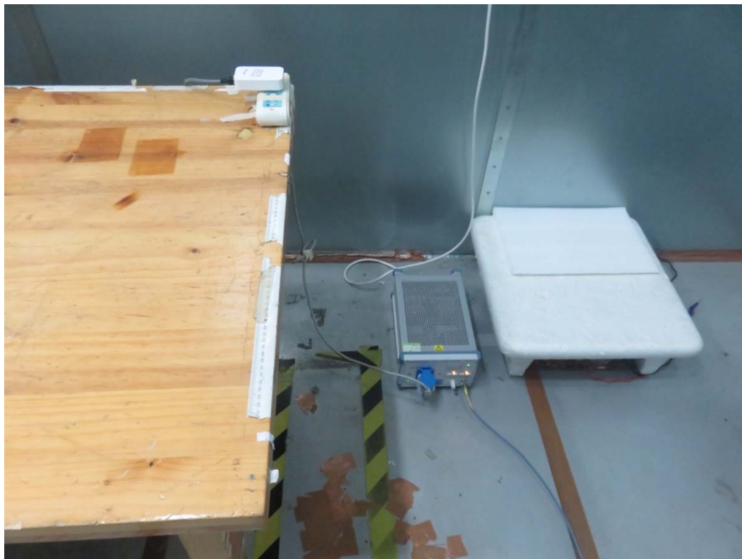
Picture 2 Conducted Emission Test Setup
