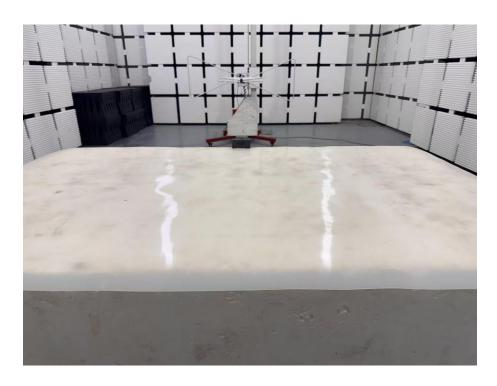
**Set-up for Radiated Spurious Emission, Above 1GHz**
