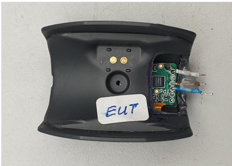
Photo 3. Test specimen with shortened programming wires. Back view.
