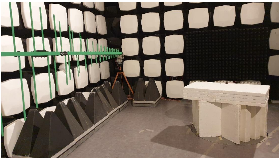
Photo 8 - Radiated emission test setup for 30 - 1000 MHz.
