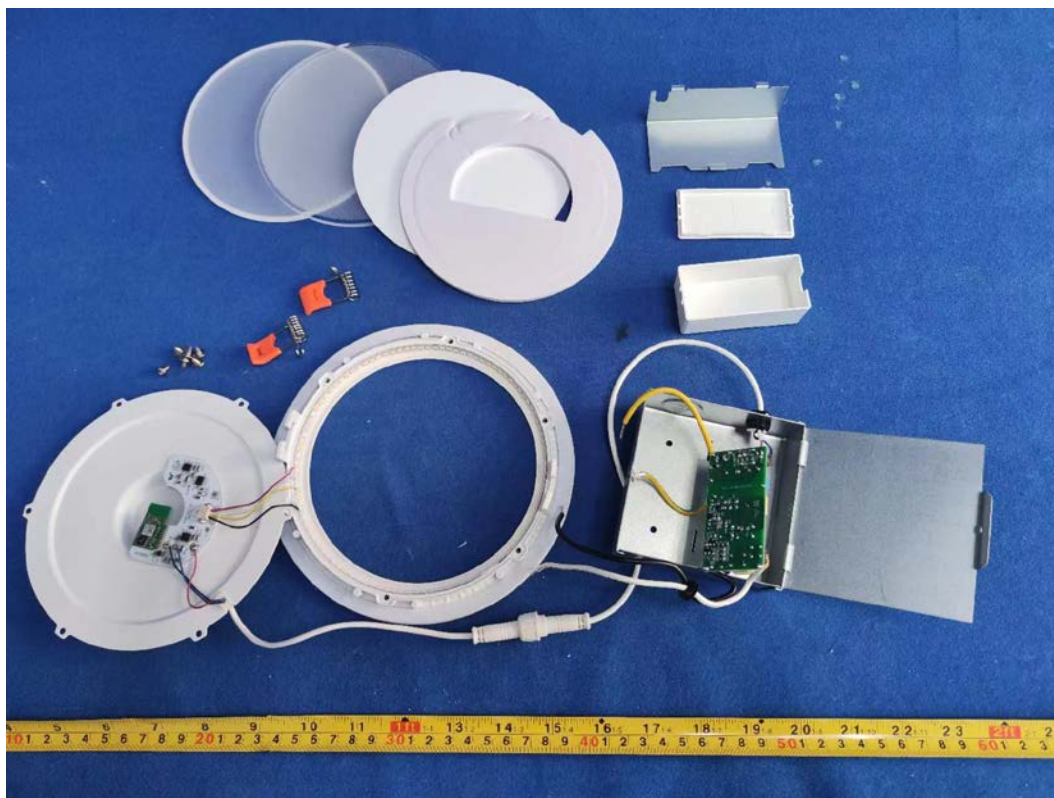
FIGURE 12 DOWNLIGHT (M/N: CFIXCNLR6S1) COVER REMOVED
