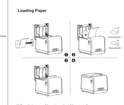
(1) Open the top cover of the printer and install the paper roll into the paper width adjuster (Figure 1); (2) Insert the roll paper as shown in the 2 illustration; (3) Pull out a part of paper, and close the cover as shown in the 3 illustration; (4) Tear off the paper with the cutter.
